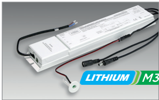
STANDARD OR SELF-TEST EMERGENCY CONVERSION PACK WITH LITHIUM (LiFePO 4 ) BATTERY - SEE PAGE 69
